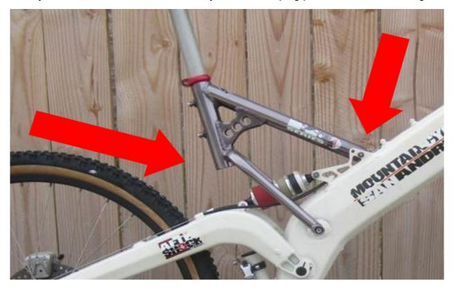
Later in the year they started to change the subframe towards the 95 model. The front clamping part lost the milled part. But the seat post tube was still cut horizontal.
