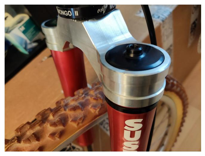
The suspenders fork crown was redesigned in the upper part. The hollow cast fork crown was replaced with a milled design
