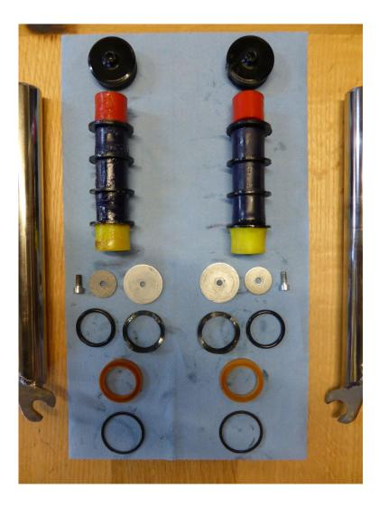
Suspender System II elastomere stack and top out spring
