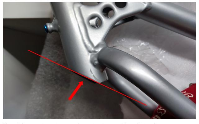
The sub frame got a cut away on the seatpost support for weight savings
