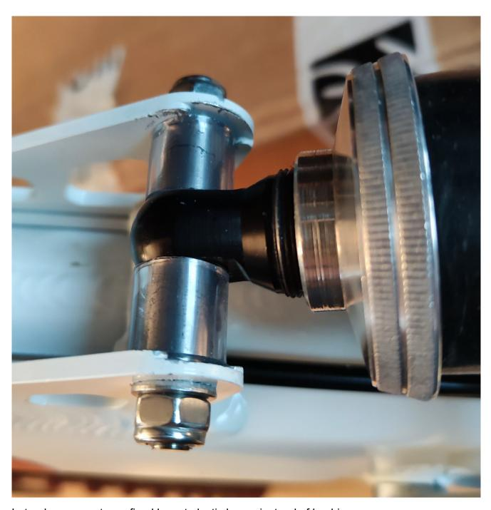
Lateral movement was fixed by cut plastic hoses instead of bushings
