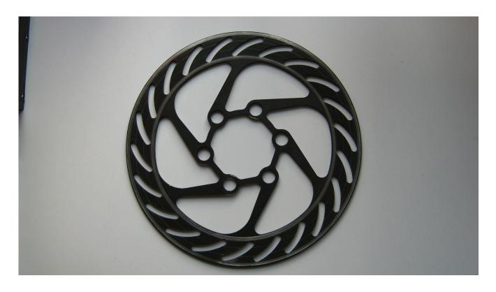
Revision of the Pro Stop discs, new with slits instead of a hole pattern
