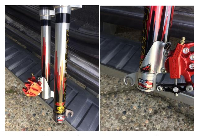
1995 Manitou EFC fork with Pro-Stop mount but with later 1996 Pro-Stop 2 mounted on them.
