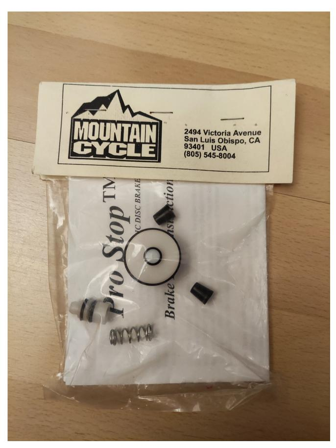
Caliper Rebuild Kit, Positive Retraction
