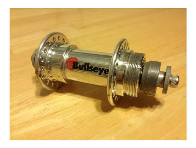
The first Pro-Stop discs used a threaded disc adapter. Hubs were Bullseye. After a few hard stops it was almost impossible to remove the disc spiders again.
