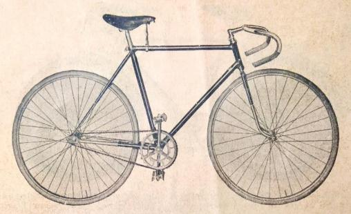
Built either for exclusive Path work with specially long draw back fork-ends or dual Path/Road with forward drop-outs, this machine is the real "goods," every ounce being utilised for propulsion. As used by several of the fastest men in the country and by an English representative at the World's Championships, 1935.
