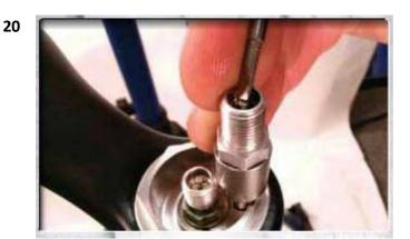
Depress the Schrader valve on the TALAS IFP tool. Again, use care when doing this so as not to get any float fluid squirted in your face or eyes.
