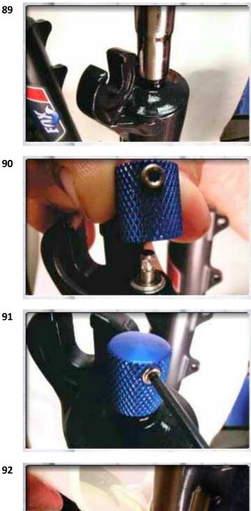
Torque the base stud nut to 50 inch pounds using a torque wrench.
