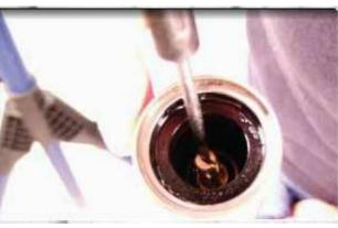
Even with most of the lower shaft slid up in the upper tube; it may not come through the top very easily. Use a screwdriver to push up on the lower shaft. Be careful not to slip and scratch any of these parts.
