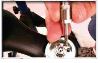
Screw the TALAS IFP tool into the IFP chamber port.
