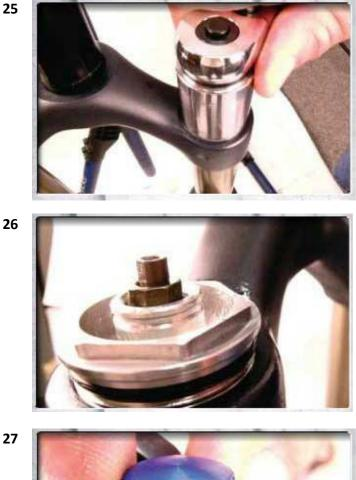
Using a 26mm socket wrench, unscrew the TALAS side top cap. Do not fully unscrew the top cap. Unscrew it enough until you can just see the o-ring (as seen in the next photo).
