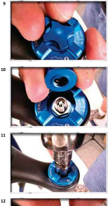
Remove the TALAS air cap from the top of the left fork leg. It can be a little tricky to grab properly. But, you can do it.
