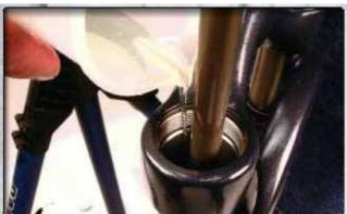
Pour 160cc of suspension fluid in the damper side top cap. Screw the top cap on by hand.
