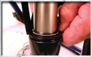
Once you have slid the upper tubes into the lower legs, use a blunt object (such as the flat end of an 8mm hex key wrench) to push the seals down into the lower legs. Press down equally on multiple sides of the seals to properly and evenly seat them.
