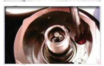
Using a small flat blade screwdriver, unscrew the red IFP port screw.
