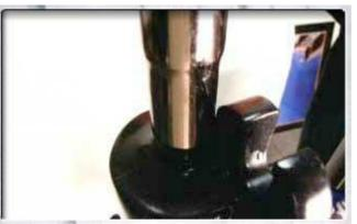
Torque the base stud nut to 50 inch pounds using a torque wrench.
