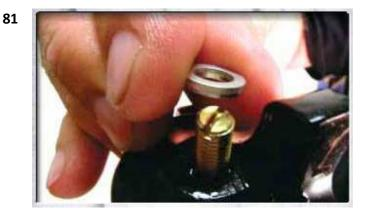
After putting in the suspension fluid, you can now push down on the lower legs until the base studs poke through the bottom of the lower legs. You may need to guide the base studs through the hole using a screwdriver to center the shaft.
