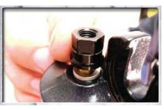
Place an aluminum crush washer on the TALAS side stud and screw the base stud nut onto the shaft.
