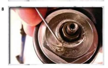
Using a dental pick or small screwdriver, carefully remove the ball and spring. Put them aside being careful not to loose them.
