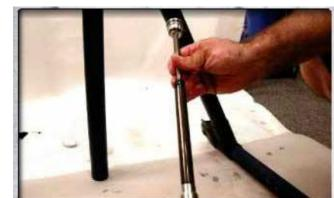
While keeping the 1.5mm hex key pushed up against the check valve, grab the damper shaft with two hands (one on the cartridge body and the other on the top cap) and pump the shaft to squeeze out any remaining suspension fluid.
