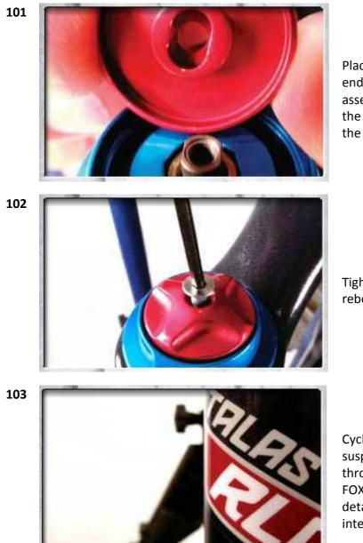
Place the red rebound knob on the end of the rebound adjuster rod assembly. Note the oval shape on the rebound knob and the top of the rebound adjuster rod.
