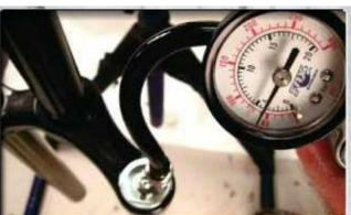
Pressurize the IFP chamber to 150psi using a FOX high pressure pump.
