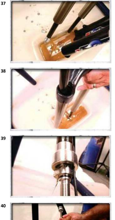
At this time you can go ahead and remove the crown steerer upper tube assembly from the lower legs. Be sure to do this over an oil pan as fluid will be draining through both sides.
