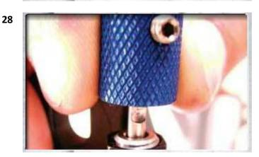
When lifting the threshold knob, notice how the set screw and the indentation on the bottom of the adjuster shaft line up. This is necessary to note when putting the knob back on.
