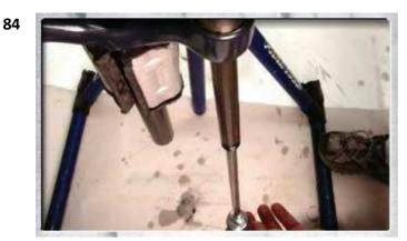
Insert the damper assembly into the right side upper tube until the base stud protrudes through the bottom of the lower leg. Throw the top cap into the upper tube a couple of turns to hold it in place.
