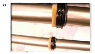
Lubricate the foam rings with suspension fluid before placing them onto the upper tubes.
