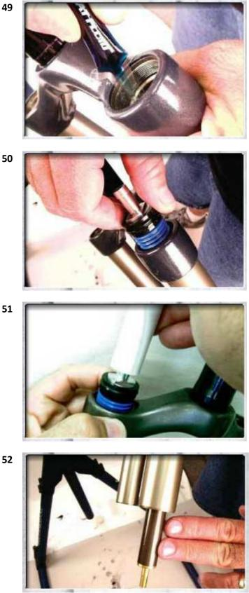
Begin reassembly by pouring 3cc of float fluid into the left upper tube. Hold the fork at an angle so the fluid does not drip out of the bottom.
