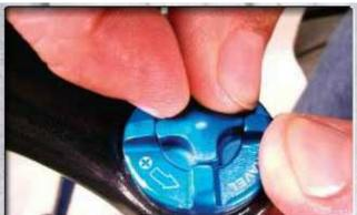
Tighten the air cap by hand.
