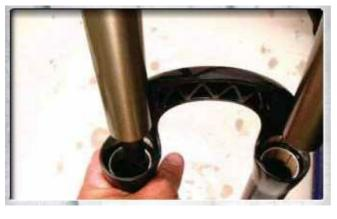
Slide the upper tubes into the lower legs ensuring that the forward crown offset is towards the fork brace. The shaft ends do not need to protrude from the bottom of the lower legs since you still need to fill the lower legs with fluid.
