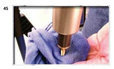
Remove the TALAS lower shaft by pushing up on the base nut.
