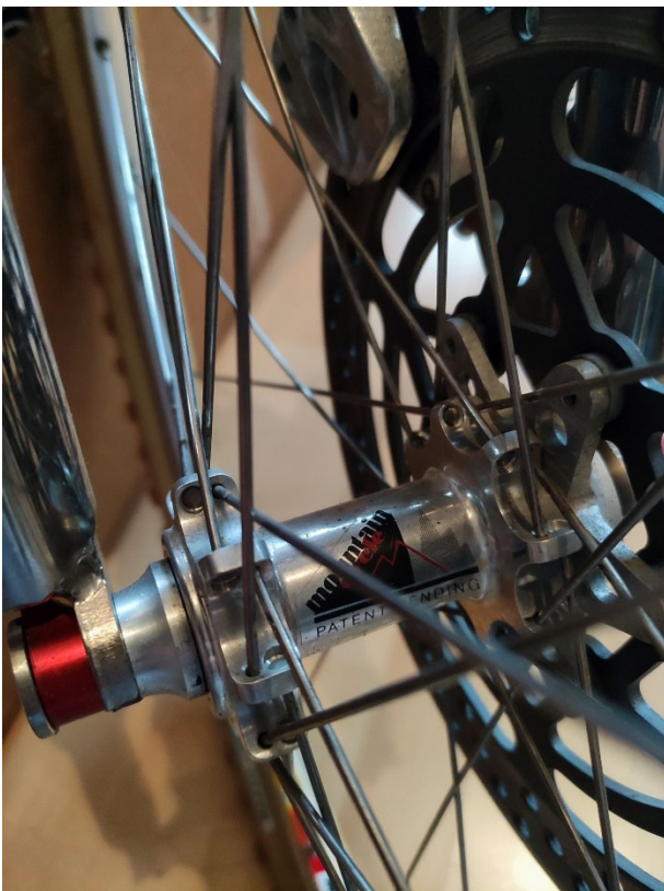
Pullstar became the new standard hub for the Pro-Stop Robert Reisinger thought that it is a nice feature to be able to replace a broken spoke anytime easily.
