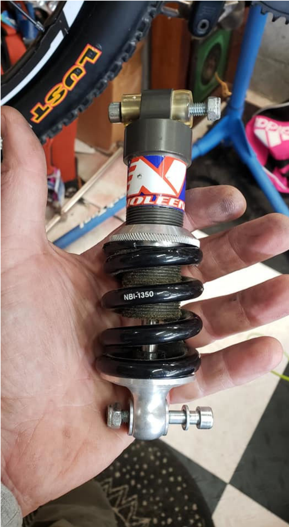
The Noleen NR1 shock allowed for longer 3" travel
