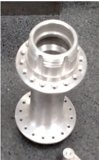
Prototype hub with the later released "wave style" rotor mount. Only a very few have been sold,
