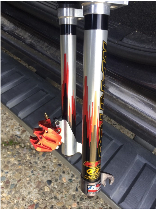
1995 Manitou EFC fork with Pro-Stop mount but with later 1996 Pro-Stop 2 mounted on them.
