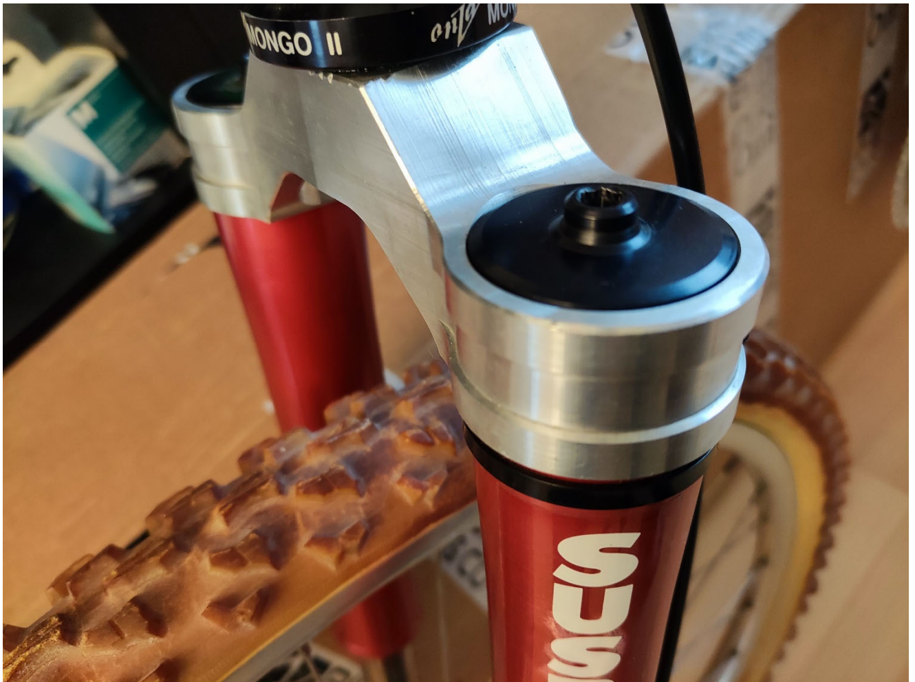
The suspenders fork crown was redesigned in the upper part. The hollow cast fork crown was replaced with a milled design
