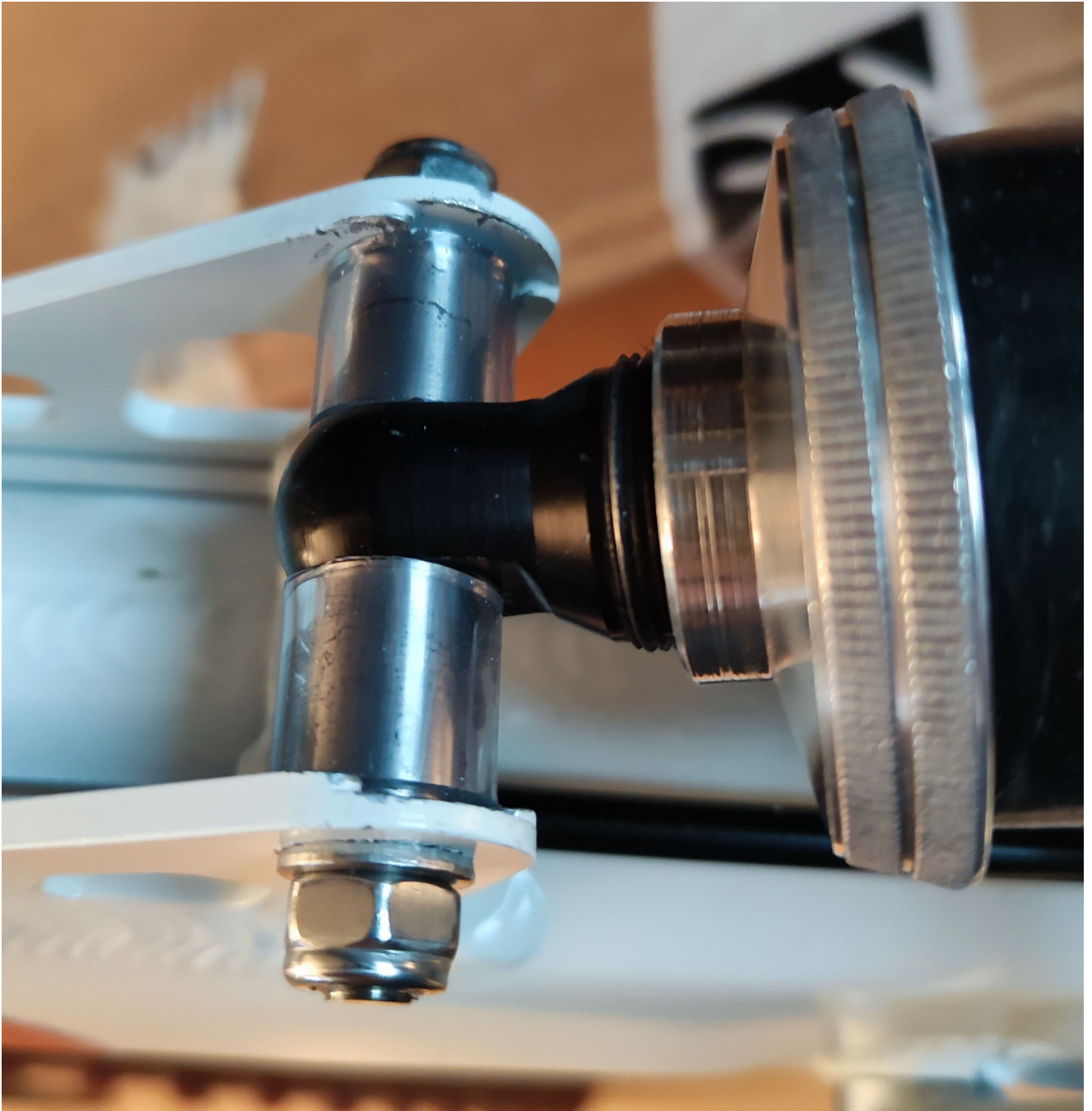
Lateral movement was fixed by cut plastic hoses instead of bushings
