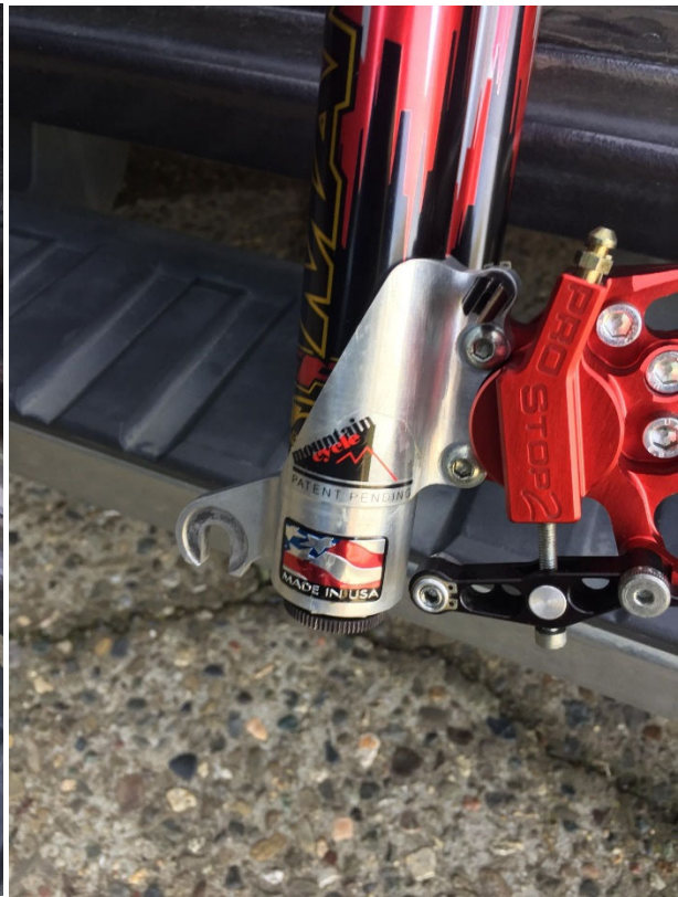
1995 Manitou EFC fork with Pro-Stop mount but with later 1996 Pro-Stop 2 mounted on them.
