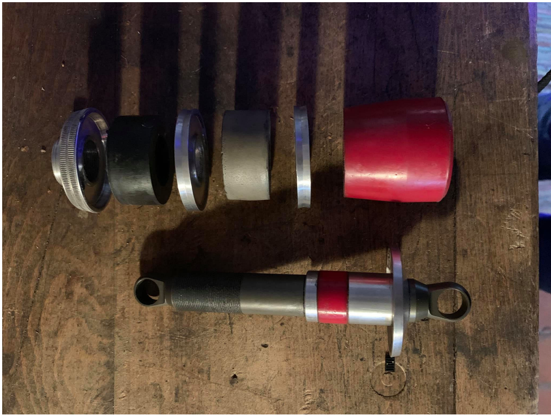
The AfterShock elastomer spring was a standard up to the 94 model. There was no damping in the shock.
